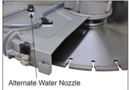
**NOTE:** There is roughly a 1mm or less effective offset (Depending on the width of the diamond segments ). Since the blade guard has some degree of flexibility, pushing down slightly brings it all the way to fully flush. In actual cutting, it comes out 100% flush. There has to be a small degree of offset so the blade won't make marks in the base material, in cases where it matters. So to avoid the marks, don't use any downforce. But to get 100% flush, use some downforce.
