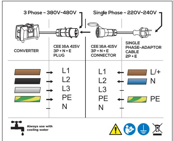
If more power is needed, and a 32A or larger breaker is available, the main plug may be removed, and the converter's main power supply cable may be directly wired to the breaker. In this case, connect the L1 and L2 wires to the breaker, leaving the L3 wire unconnected. Then connect the earth (ground) wire to the earth connection.
