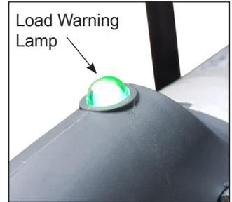
**NOTE: When using single phase 16A power, the operator must be very careful not to use too much force. One must make note of the load warning lamp and try to keep within the green range. Too much load will draw too much current and easily trip the supply circuit breaker.**
